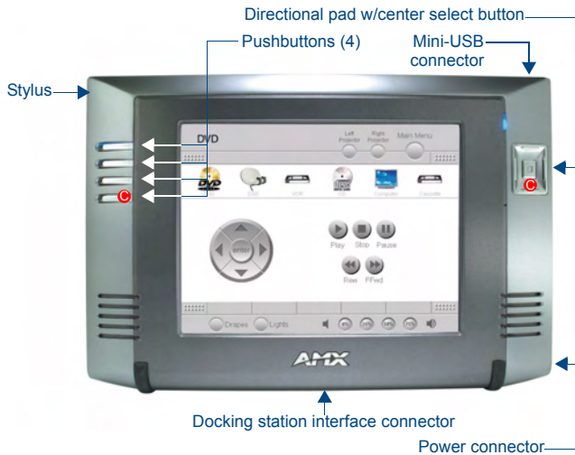
FIG. 1 MVP-7500 Touch Panel components
